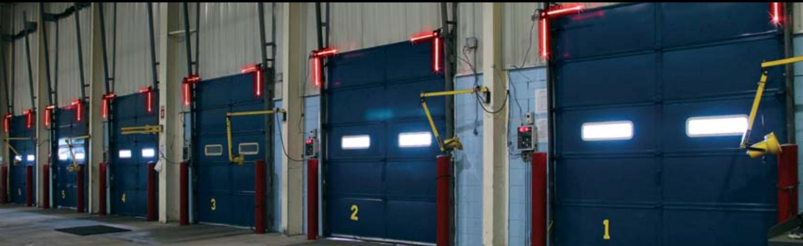
Dok-Lok restraints with Corner-Vu and Leveler-Vu lights improve safety and increase efficiency with clear communication.
